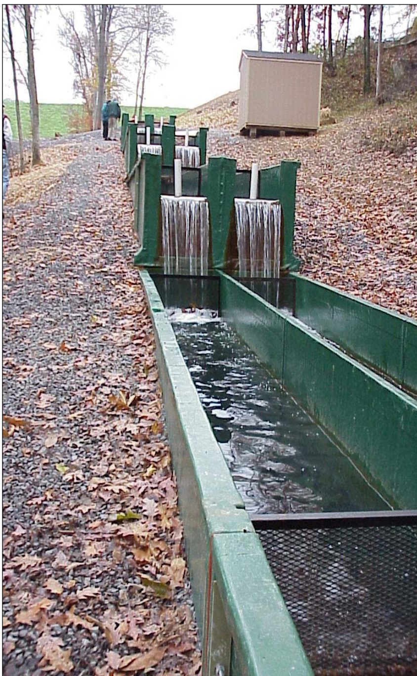
West Virginia University's research raceways use a lightweight experimental material.
