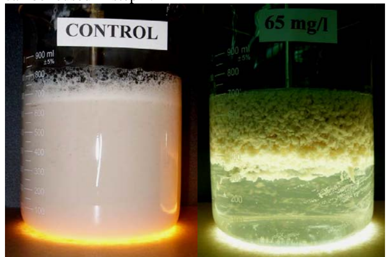
Picture 3. Protein flocculation can further enhance separation of the fish muscle proteins in the decanter-centrifuge in the recovery system. On the left are fish muscle proteins without flocculant. On the right are muscle proteins following 10-min reaction with commercially available flocculant. The optical density of the effluent water (bottom right) is comparable to that of clear water, and therefore, the water can be re-used in the recovery system.
